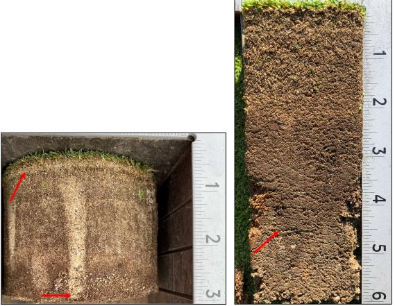
The left profile is from 17-G this year while the right profile is from 17-G last year. The profile picture from #17 this year indicates that aeration holes are being effectively filled and that there is a significant amount of sand in the upper 0.25" like 2017. This is an excellent
